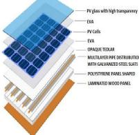
MULTILAYER PIPE DISTRUBUTION WITH GALVANIZED STEEL SLATS POLYSTYRENE PANEL SHAPED LAMINATED WOOD PANEL
